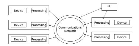
Fig. 1. Collaborative control architecture. Each intelligent hardware unit (IHU) is composed of an hardware element, processing resources and communication capabilities.
