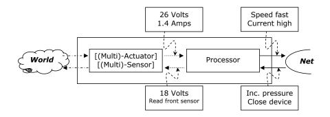
Fig. 2. Working methodology for a certain intelligent hardware unit (IHU).
