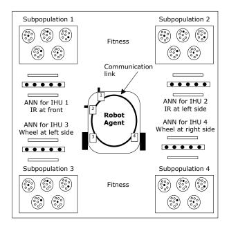
Fig. 3. Architecture for a robotic pet controlled by four IHUs.
