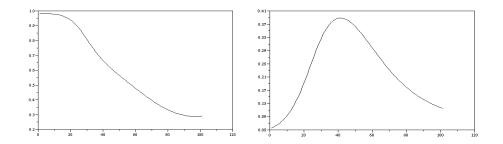
**Fig. 4.** ANN output learned by the IR sensor X. Because function depends on 4 variables, sensor Y, Left motor and Right motor have been fixed, showing only the dependence of the network output in front of sensed X values.
