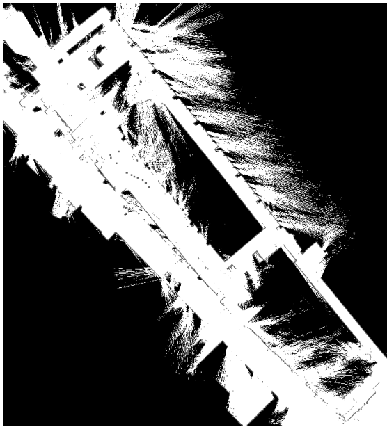
Figure 2. Automatic loop closure failed in the left-upper part of the map (size of the loop 50x10m). At the same time, debris due to ephemeral obstacles can be observed in the main corridor.
