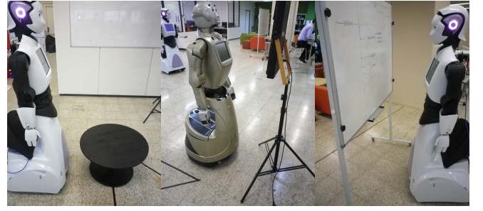
Figure 4. Different types of objects that we have encountered in the deployment of our robots Reem-H and REEM, that are difficult to be detected (a small table, the foot of a light projector and a white board).
