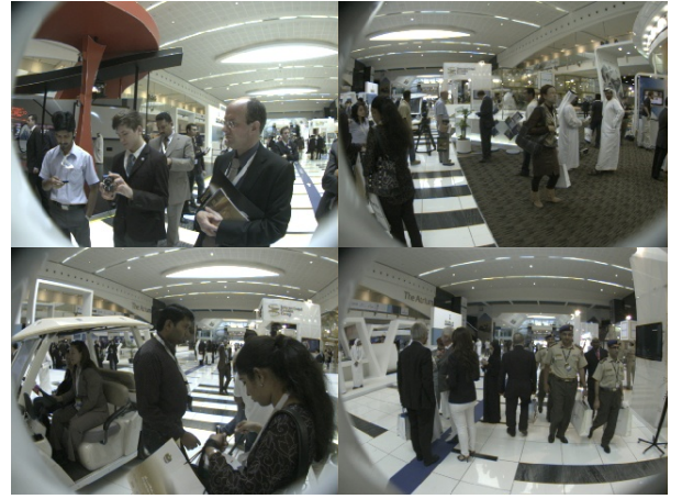
Figure 3. Four different images obtained by REEM robot at IDEX exhibition (its head in normal operation position). It can be observed that a large amount of visual localization information can be obtained by paying attention to the signs at the upper part of the images, which is almost never occluded.
